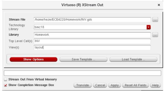
**Note**: Make sure the Technology is "tsmc18" since this tutorial is based on TSMC 180nm technology.
