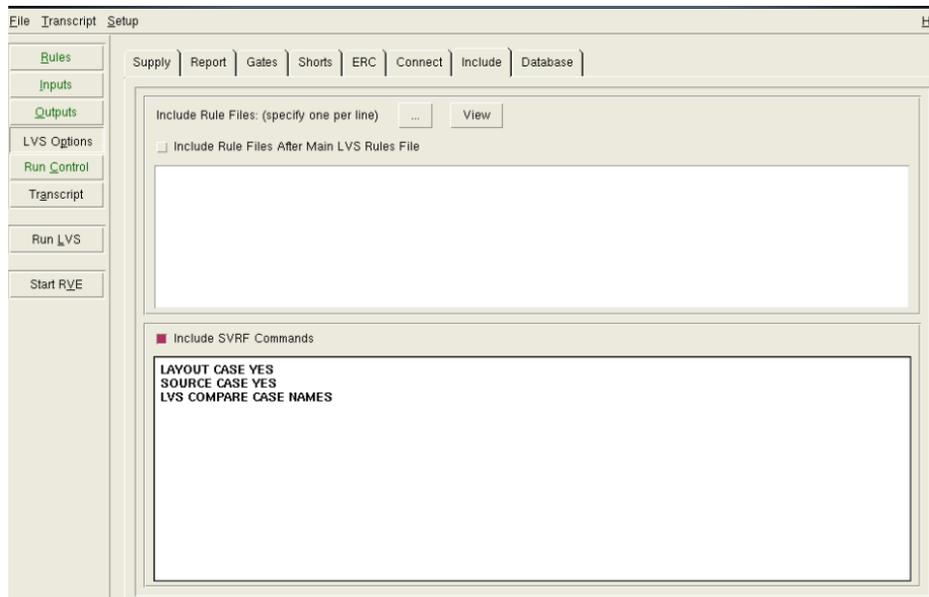
6. Go to **Supply**, for **Power nets**, enter **VDD**; for **Ground nets**, enter **VSS** (case sensitive).
