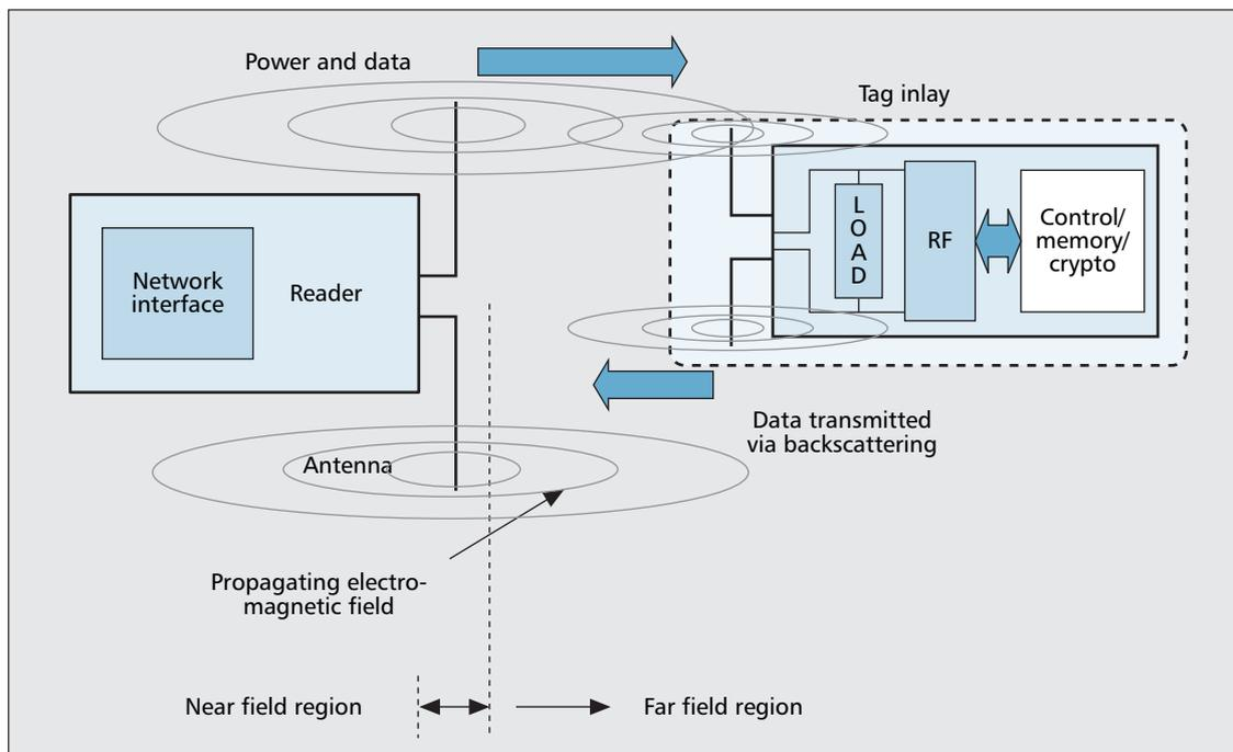
■ Figure 4. Far-field communication via backscattering.
