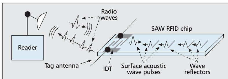
■ Figure 6. Operation of SAW tag [adopted from [www.rfsaw.com/tech.html](http://www.rfsaw.com/tech.html)].
