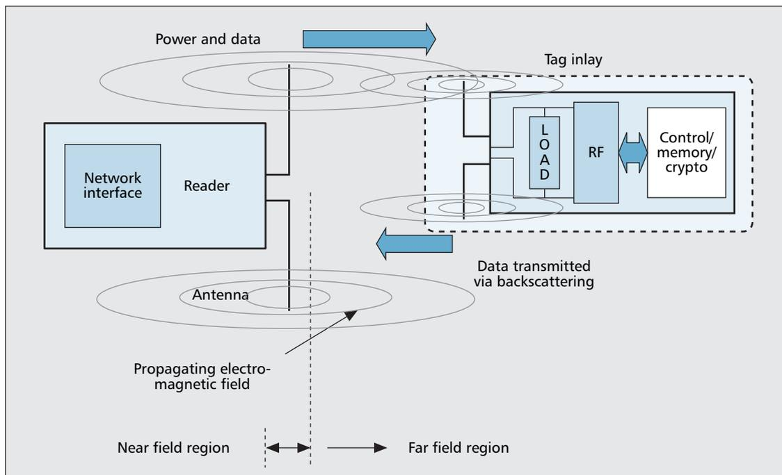
■ Figure 4. Far-field communication via backscattering.
