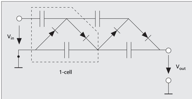
■ Figure 1. Two-stage Greinacher half-wave rectifier [2].
