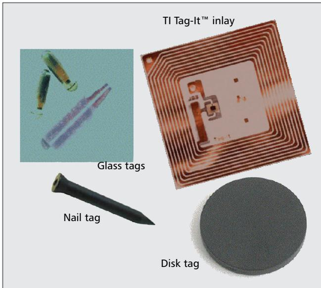
■ Figure 3. Different types of near-field RFID tags.
