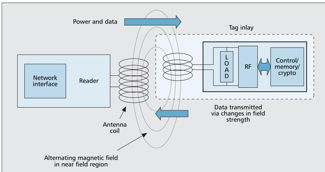
■ Figure 2. Near-field communication using inductive coupling.
