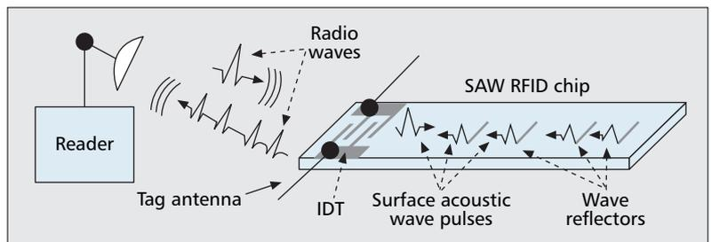
■ Figure 6. Operation of SAW tag [adopted from [www.rfsaw.com/tech.html](http://www.rfsaw.com/tech.html)].
