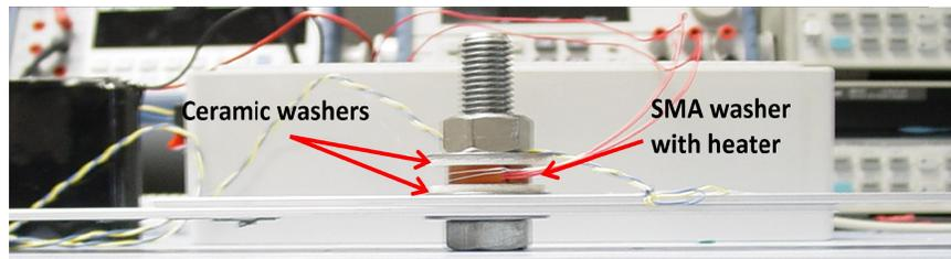
Figure 9: SmartJoint with an External heater
