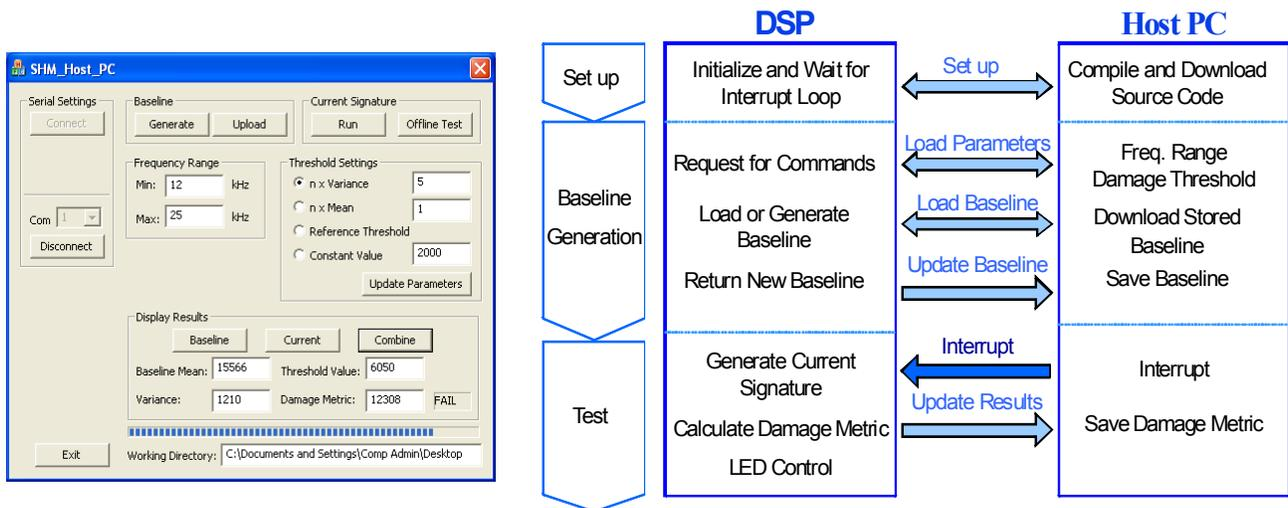
Figure 7: The GUI and the Test Flow for Our SHM System
