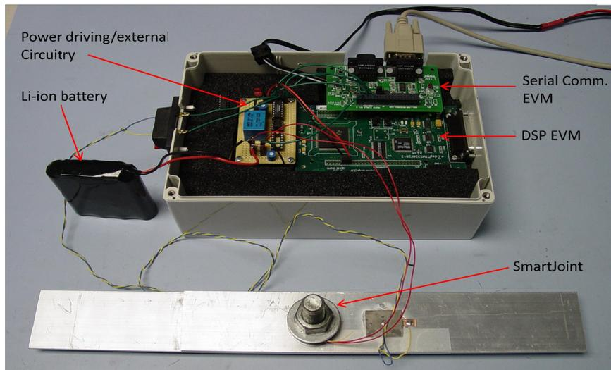
Figure 8: System Setup
