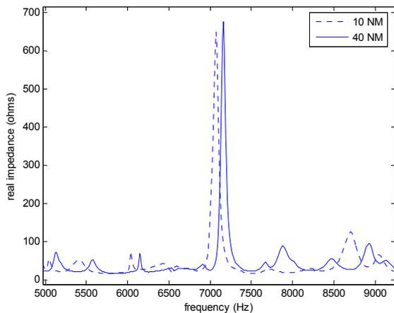
Figure 4: Impedance Profile of a SmartJoint
