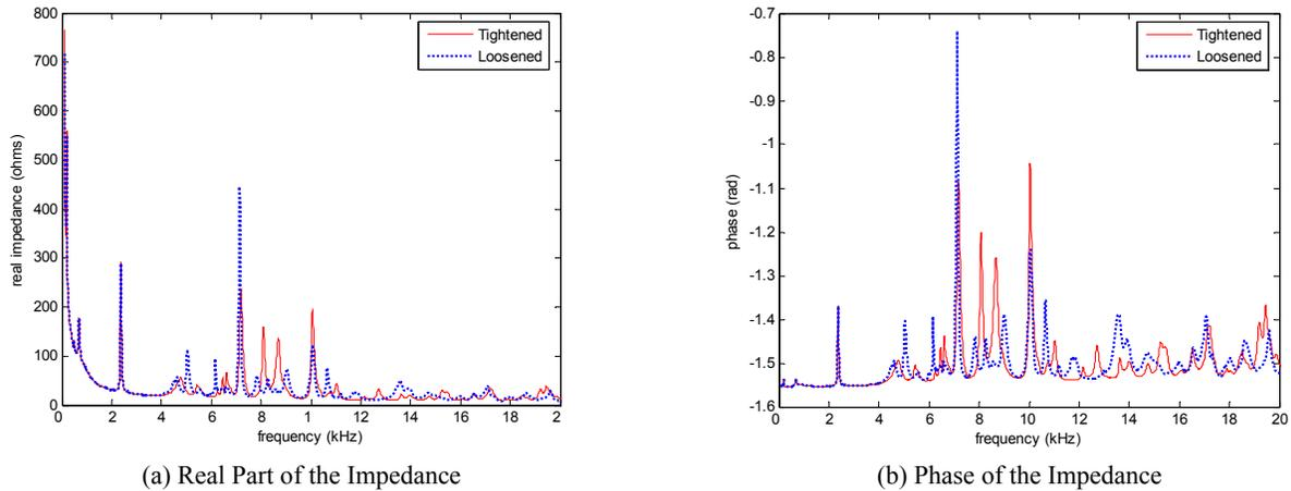
Figure 10: Impedance of the SmartJoint
