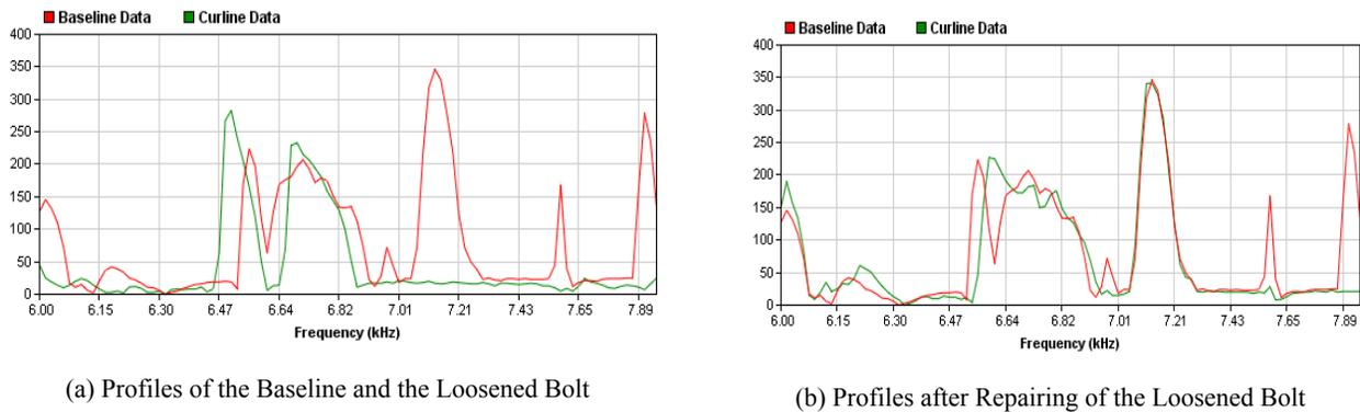
Figure 11: Profiles of the Baseline and the Loosened Bolt Before and After the Repair
